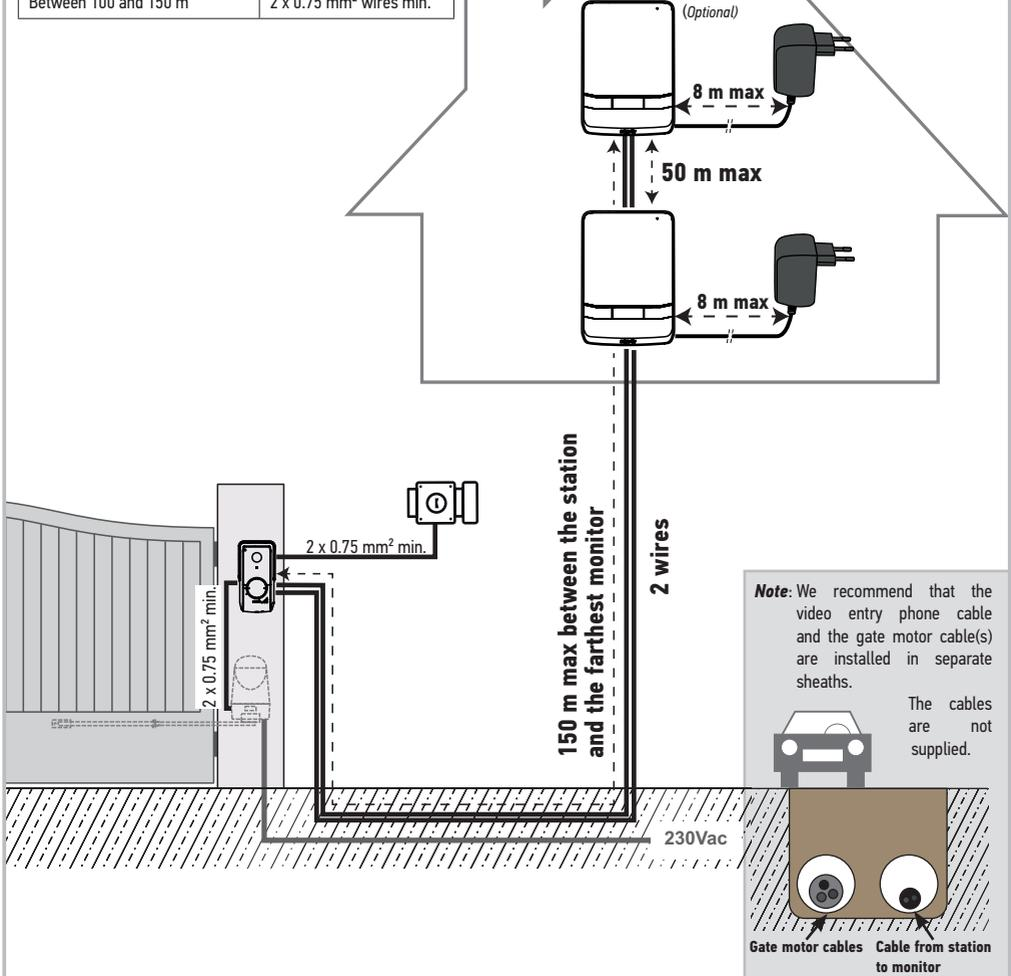
**Note:** If you need to use junction boxes to cable the video entry phone, do not use more than two boxes between the station and the monitor, or more than one box between the monitor and the power plug.
